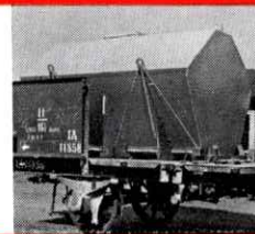
Bulk cement container. Ply-wood construction.
