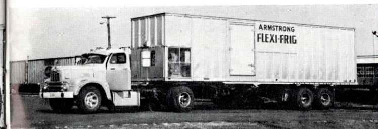
Flexi-Frig container, for perishable goods, with automatic diesel engine powered freezer unit (Flexi-Van system).
