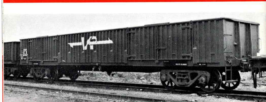
ELX open wagon. Two sets of double-hinged doors both sides without stanchions. Fluted sides for partitioning loading.
