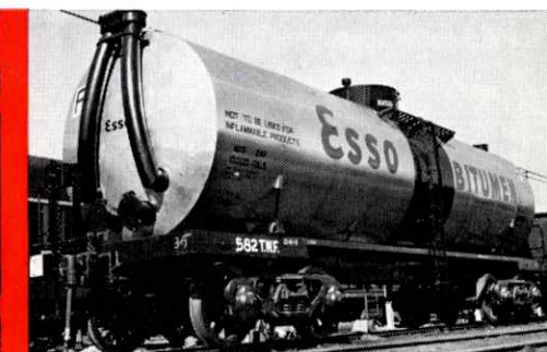
Bitumen tanker with heater tubes.
