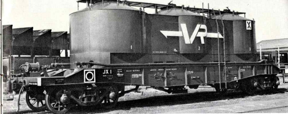
JX bulk cement wagon. Gravity fill and pneumatic discharge.
