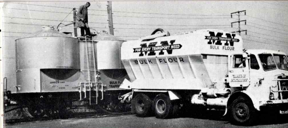
FJ bulk flour wagon. Gravity fill and pneumatic discharge.
