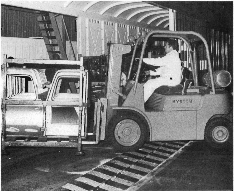
BELOW: Giving an idea of the great size of the new high cube vans, this fork lift loads up at Broadmeadows. The 39 vans will carry vehicle parts previously carried in 160 conventional wagons.
