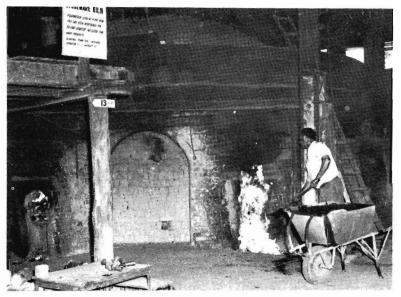
Once the peak temperature is reached, the kiln is fired four times with salt—at two hourly intervals—to set the glazing. The kilns are then sealed and left to cool.
