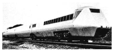
The gas turbine powered prototype Advanced Passenger Train. It is designed for speeds of up to 155 m.p.h.  $(250~km\,/h)$  on existing tracks and to exceed 200 m.p.h.  $(322~km\,/h)$  on the new tracks.
