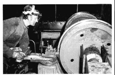
Fitter and Turner Barry Ward uses Ballarat North Workshops' mimic lathe to turn a set of wheels. This lathe was specially adapted for this duty. Barry, who has been with the V.R. for 17 years, spent eight years at the Newport Workshops before transferring to Ballarat.
