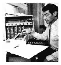
Lighting and Power Design Engineer, Don Rowe, indicates the PROM memory banks inside the brain box of the electronic train destination board controller. The memory banks control the five output switching cards in the control box behind Mr. Rowe's hand.
