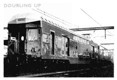
Sydney's new eight-carriage double-deck metropolitan trains (above) are now coming into service. Carrying 2,104 passengers, seating capacity is improved by over 90 per cent compared to the older single-deck trains. Each of the 12 complete trains will cost \$1.3 million. A further order of double-deck trains has been placed for the Eastern Suburbs Line now being built.
