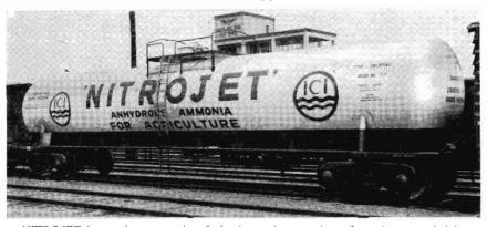
NITROJET is another example of the increasing number of products carried in specialized rail freight vehicles. This liquefied ammonia is railed from Port Kembla to Yarraville for Imperial Chemical Industries of Australia and New Zealand Ltd.
