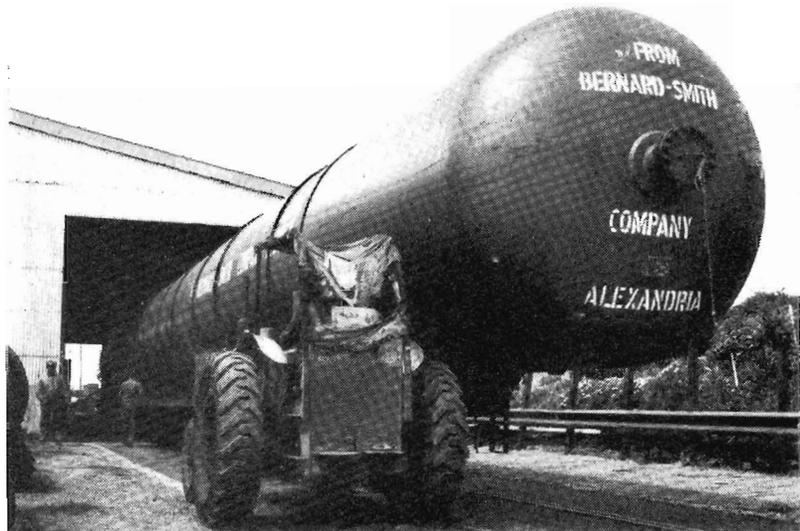
**BIG LOAD :** Typical of the railways' ability to handle any kind of traffic, was the transport, last month, of five huge pressure vessels from Cooks River, N.S.W., over the standard gauge line to Dynon Bogie Exchange, and thence to Western Australia. Each pressure vessel was about 108 ft. long, 10 ft. high and 48 tons weight.
