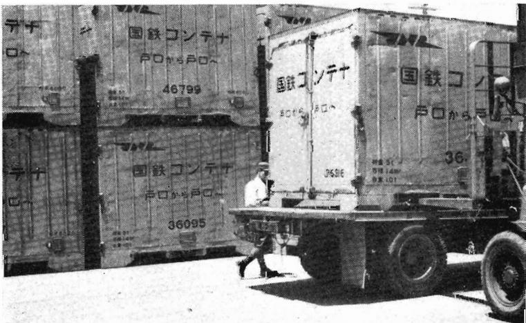
Standard containers at Umeda Yard, Osaka. These are 10 ft. 9 in. x 7 ft. 9 in. x 7 ft. 9 in. with doors at one end only. Note loading by fork lift truck. It will be seen from the dents that the containers must be robust to withstand normal usage.
