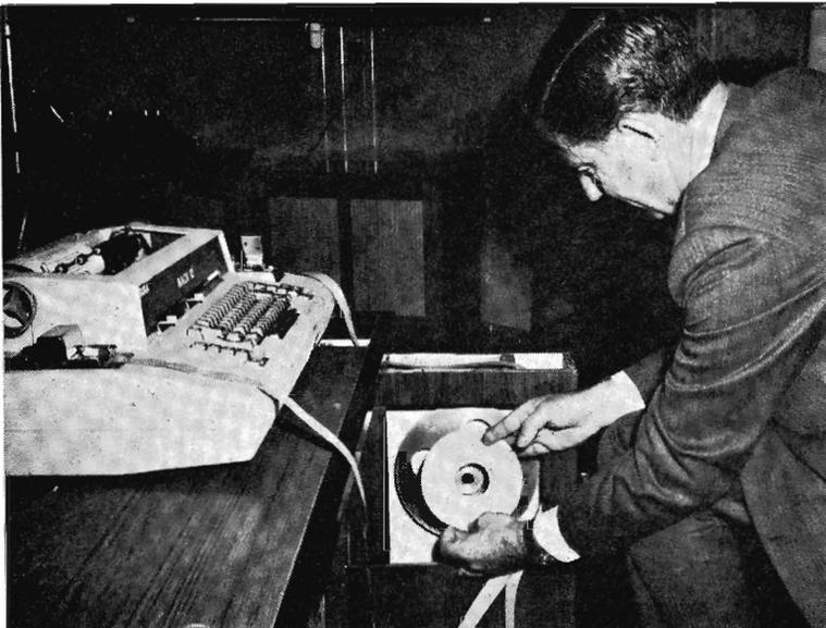
Mr. L. Lynch, Controller, Management Services Division, loads paper tape into container. Tape at left of machine feeds into the photo-electric reading unit; tape at right feeds from the punching unit.
