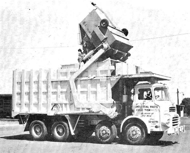
Contents of the container are emptied into the packer body where it is compressed by a hydraulically-powered packer plate.
