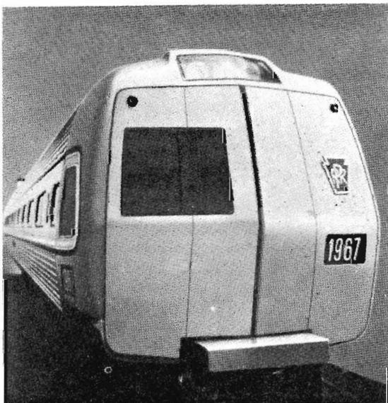
Mock up of a self-propelled, electrically driven, multiple-unit rail-car ordered by the Pennsylvania Railroad Co. to attract passenger traffic for its New York-Washington service. Fifty will be required at a cost of over \$US400,000 each.
