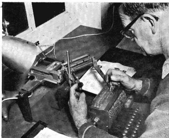
Engraving passenger's name on a ticket. One end of the pantograph holds a pointer with which the operator is tracing the letters cut on the brass copy drum. The other arm of the pantograph holds a diamond point that, in reduced size, does the engraving. The drum was designed and made at the Workshops.
