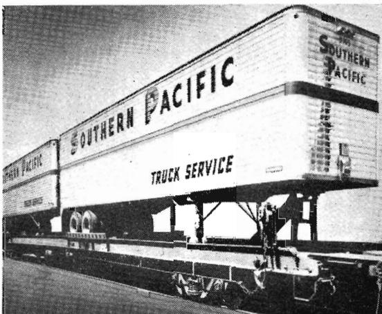
Piggy-back wagon showing retractable trailer hitch supporting front end of road semi-trailer.
