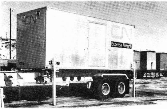
C.N.R. standard 20 ft. container on temporary legs so that road transport may be positioned under it. This type of container is usually loaded by a side loading unit.
