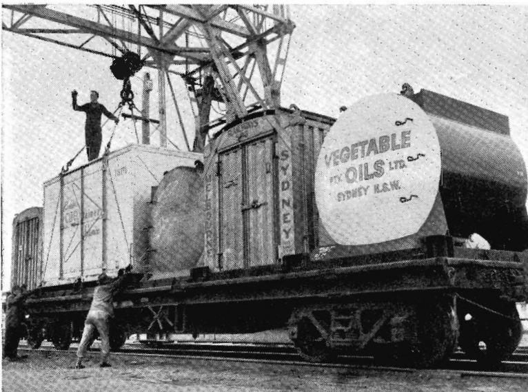
Loading containers at Dybon. The container system takes advantage of the ability of highway vehicles to go anywhere there is road access, and the railway's ability to move full unit loads with speed and economy.
