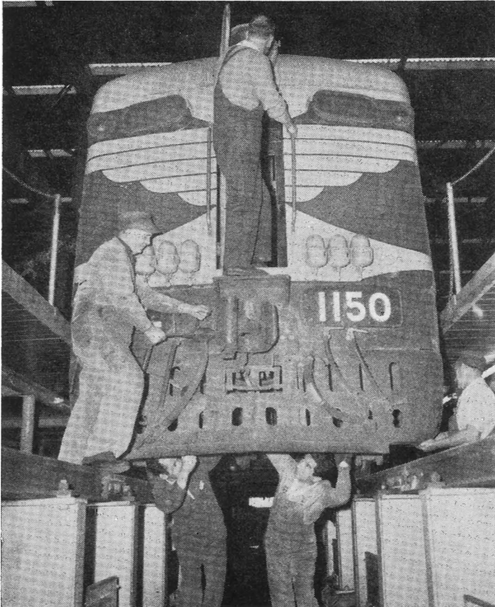
MAINTENANCE of electric locomotives is now being done at South Dynon Loco Depot. L. 1150, the first electric main line locomotive that was bought by the Department, is shown undergoing one of its regular inspections.
