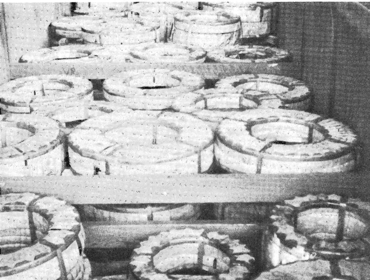
These coils of strip steel are in an ELF wagon that has been fitted with 8 in. by 3 in. wooden divider beams to carry special types of loading that need this protection during transit. It is the first of a group of wagons to be fitted with the beams. The steel strip from Port Kembla, is going to Geelong.
