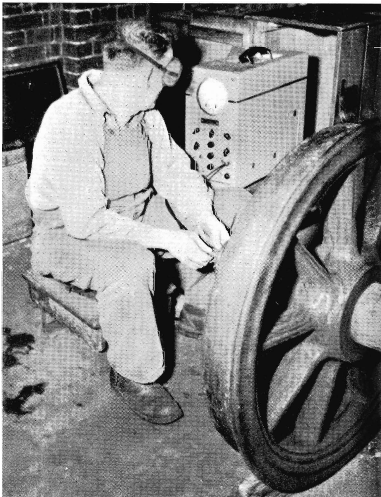
Testing an axle with an ultrasonic flaw detector. Such testing has proved of considerable value in preventing service failures and costly derailments.
