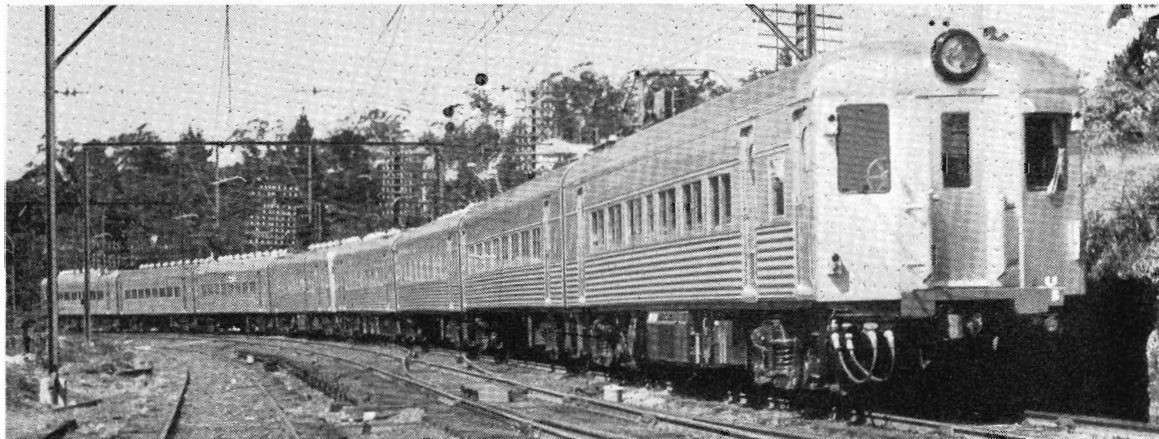
A stainless steel inter-urban electric train of the type used on the service over the Blue Mountains to Lithgow, and north to Gosford. NSWGR has 80 of these cars in service. They are operated in units of four, six or eight cars.
