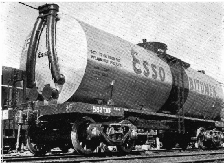
Stainless steel tanker for bitumen is another specialized goods vehicle.
