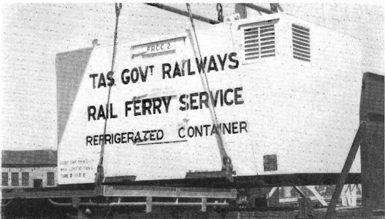
Refrigerated Container F.R.C.C. type, used on Rail Ferry Services. Maximum load 10 tons, cubic capacity 55 tons.
