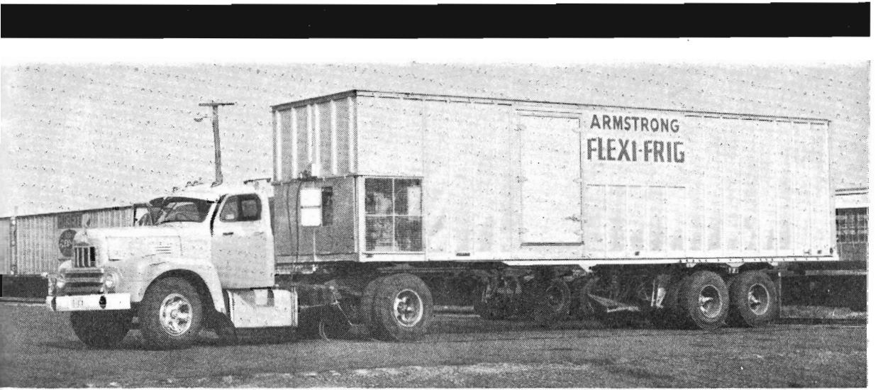
FRIG : A new variation of the Flexi-Van rail-road co-ordinated transport went into service last month. With a completely self-contained refrigeration unit it is intended for the transport of such commodities as frozen vegetables, cheese, margarine, ice-cream and fish. The Flexi-Frig is 35 ft. long, and will carry up to 20 tons. It is transferred between the road vehicle and the special rail wagon in the same manner as the ordinary Flexi-Vans and Flexi-Flats.
