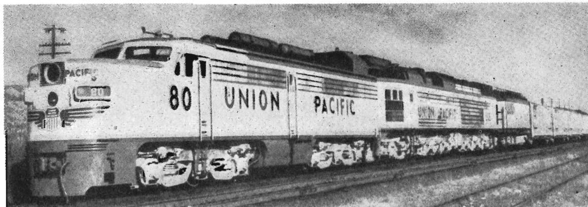
The world's first direct-fired, coal-burning gas turbine-electric locomotive which is undergoing road tests on the Union Pacific railroad (America). Designed and built by Union Pacific, the complete locomotive is rated at 7,000 h.p. It consists of a 2,000 h.p. diesel-electric unit, a 5,000 h.p. coal-fired gas turbine unit and a tender which carries coal pulverizing equipment and coal. Total length of the two units and tender is 215 feet. ( Railway Age )
