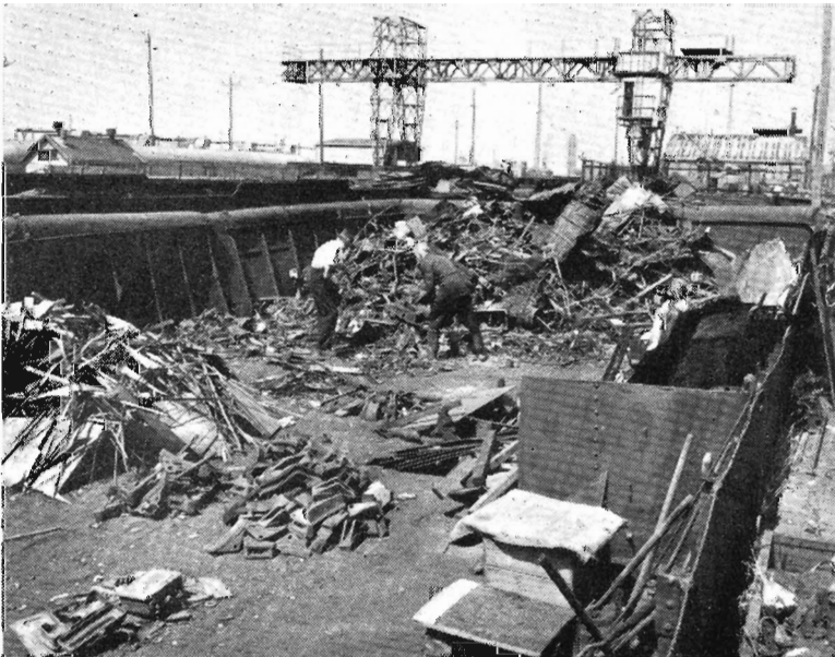
In the sorting bin, ferrous scrap is sorted into various classifications, such as cast iron, small steel, pressings, etc.
