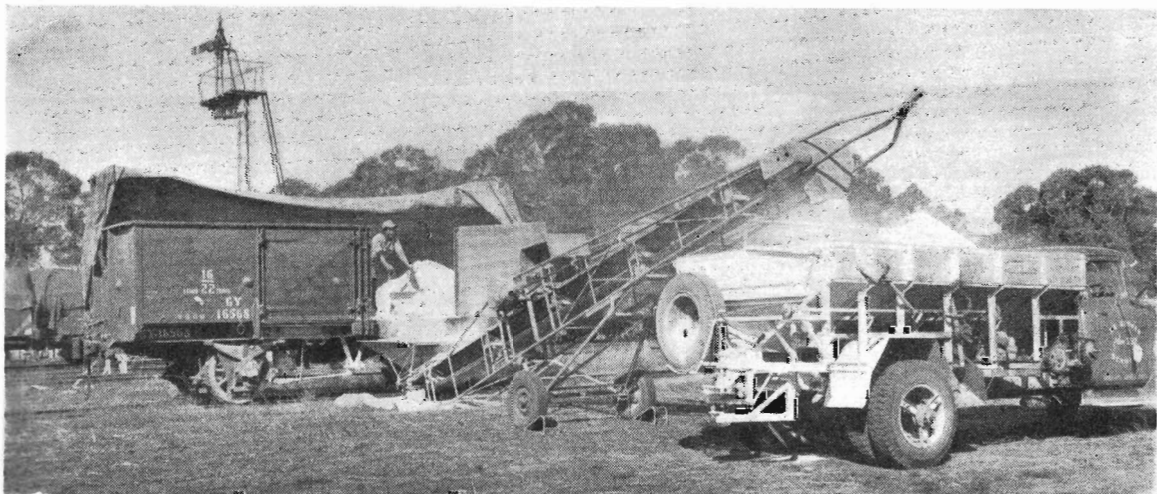
At Glenorchy, a 6-ton hopper-spreader road truck is loaded in 15 minutes direct from rail wagon. After the truck spreads the fertiliser on local farmers' land, it returns for another load.
