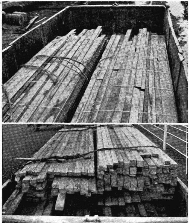
Showing the loading system in operation. (Above): Two bundles are laid on truck floor. (Below): Two further bundles are placed above them, bringing the truck's total tonnage to 12.
