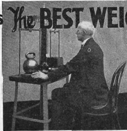
Foreman W. Turner, who has charge of V.R. scales, testing one of the railway check weights with the Department's copy of the Imperial Standard Weights.
