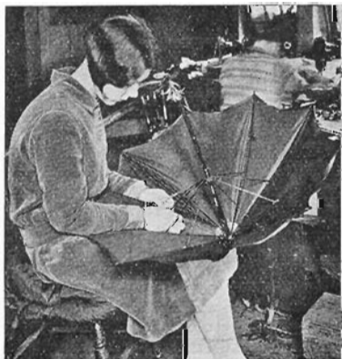
Tying in the seams of the sections of cloth against the ribs
