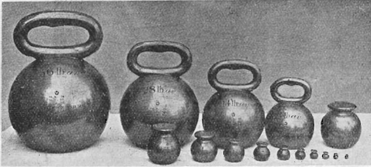
The Victorian Railways copies of the Imperial standard weights. These copies check all weights used on Victorian railway scales.
