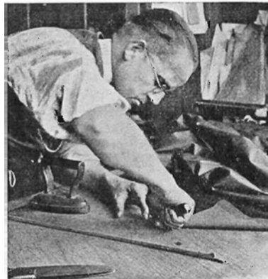
The beginning of an umbrella. The cutter runs his knife round a template on the cloth
