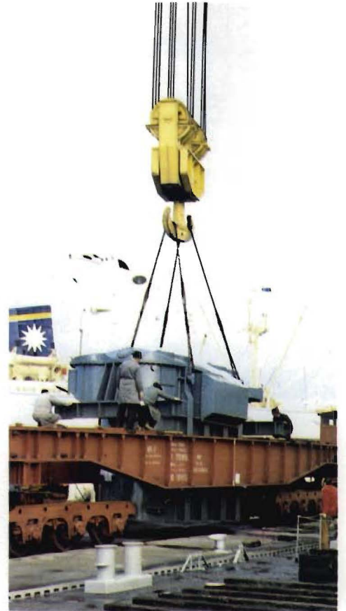
Victorian Railways has special wagons for heavy commodities such as this transformer for the Latrobe Valley.
