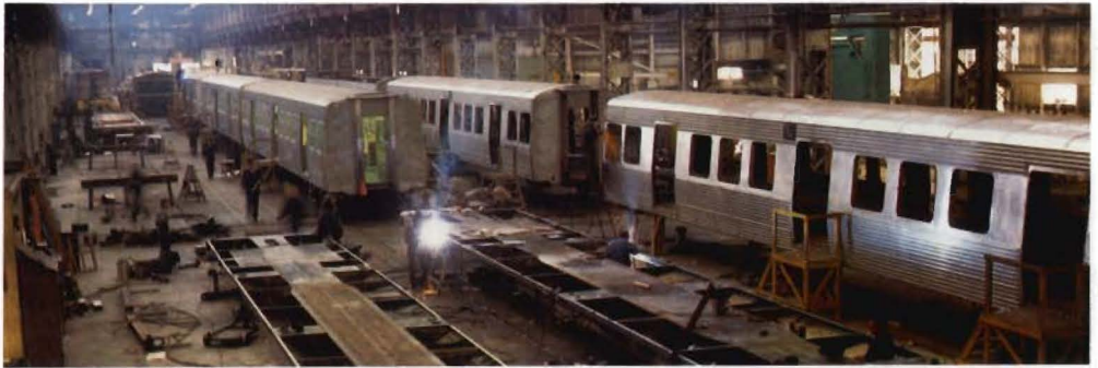
Stainless steel suburban train trailer carriages on the production line at Newport Workshops.
