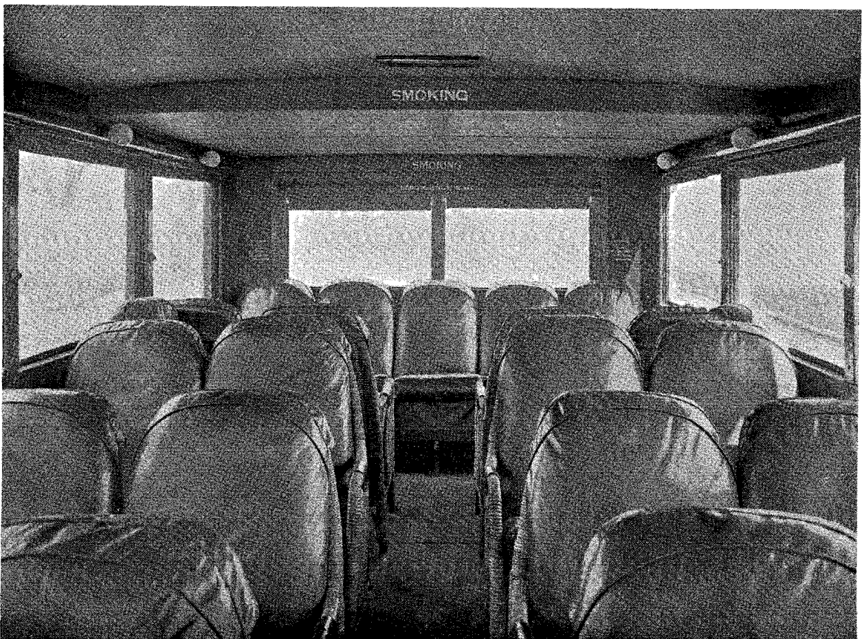
INTERIOR VIEW OF "INTERNATIONAL" 23-PASSENGER SEDAN MOTOR COACH, SHOWING SEATING ARRANGEMENTS, Etc.
